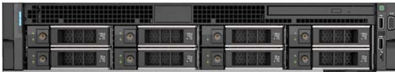
R740 Front view - 8 x 3.5" hard drive configuration
