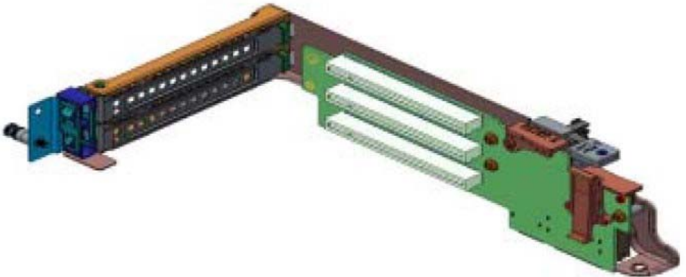
Riser 2B - 1 slots, 1x8(Top and bottom)
