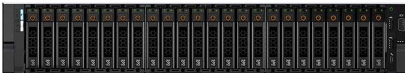
R740xd Front view - 24 x 2.5" hard drive configuration
