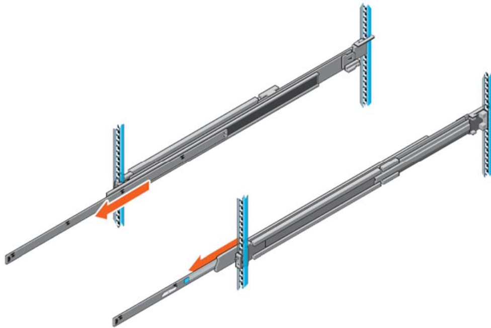
Figure 18. Pull out inner rail
